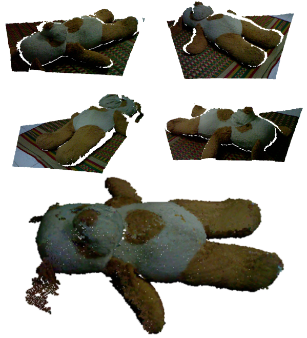
Figure 9. Four input point clouds corresponding to four viewpoints and the pairwise-registered point cloud (bottom)
