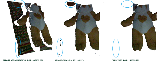
Figure 3. A point cloud before segmentation, after segmentation and after clustering
